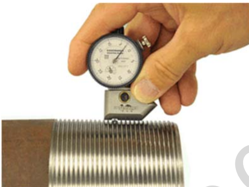
TA-3002 Thread Addendum Gage Inspecting a Part
